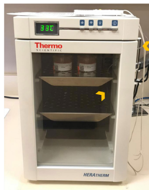
Figure 1A Heratherm™ Compact Microbiological Incubator. Two corneas inside of their viewing chambers can be seen through the clear door. The orange arrowheads show where the temperature probe for active monitoring is located inside of the incubator (bottom arrowhead) and where it exits the incubator.
