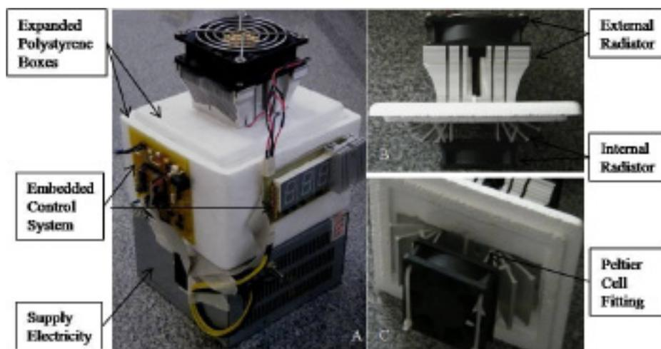
FIGURE 2. Prototype box for corneal transport. A: external view; B: prototype cover; C: Peltier cell fitting.
